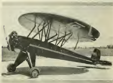
Nemuth parasol-type monoplane powered by a Warner Scarab engine of 110 h.p.
